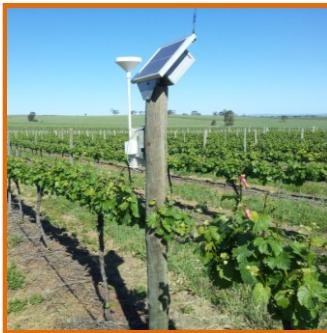
*One of four Model T MetStations maintained by CWRGA to collect and transmit weather data. This one is at Auburn. These stations provide data to improve decision making, particularly in relation to downy mildew infection events. (Photo: David Olssen)*
